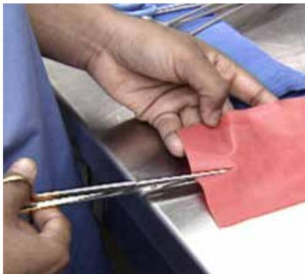
Figure 2– Function Test for Sharpness of Scissors
